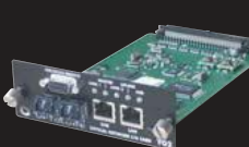
OPTOCORE YG2 16 channel Optocore I/O
