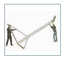
Start lifting the mast in place, until reaching the vertical position.
