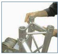
Place the Lift Base on the ground and lock the stabilizers. Unroll about 7 mt of the steel cable.
