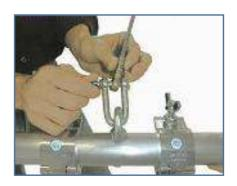
Lock the flying bar and the steel cable, by using the specific shackle.
