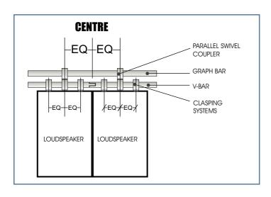
Placement of the adjustable V-bar for two loudspeakers (TB 9576).
