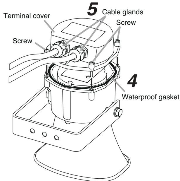
**Step 7.** Securely tighten the cable glands.
