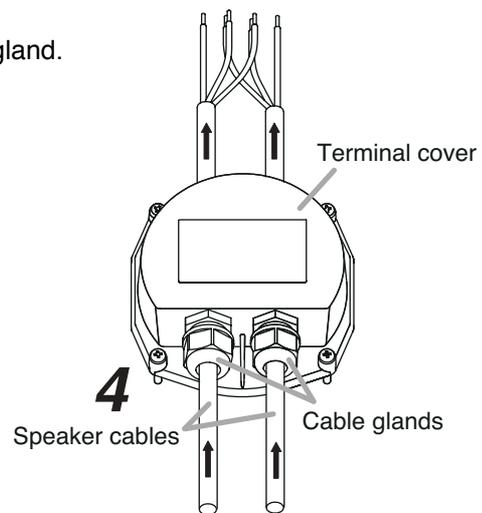
**Step 5.** Connect the speaker cables with the same polarity to each terminal according to the polarity indication at the screw terminal.
