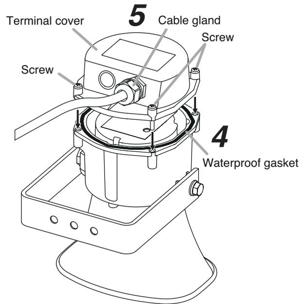
**Step 5.** Securely tighten the cable gland.
