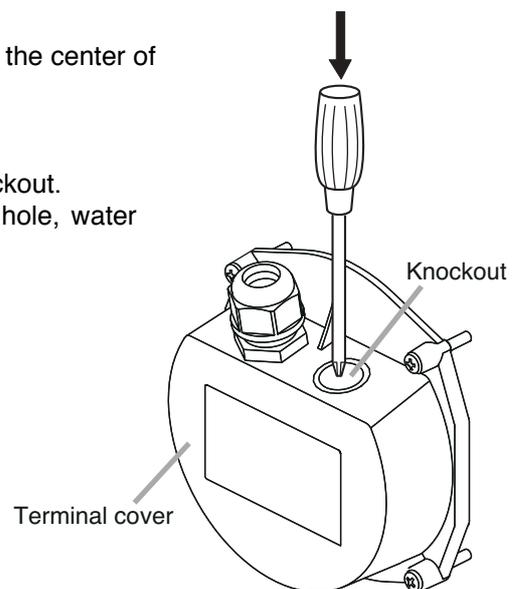
**Step 2.** Attach the cable gland to be added.
