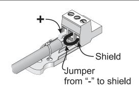
**Unbalanced inputs can be used if required.** If unbalanced audio sources are used, it is preferable to use an appropriate audio transformer (or other unbalanced-to-balanced "converter") to provide a balanced input to the DSP-3. If this is not possible, then it is recommended that the negative terminal and shield terminal be connected to one another with a jumper wire.
