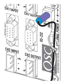
Insert the coaxial power plug into the EXTERNAL POWER jack. Ensure that the plug is firmly seated in the jack. Use the "tab" provided on the chassis for securing the power cord with a tie-wrap (wire-tie).
