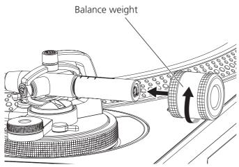
If a horizontal balance cannot be obtained because the cartridge is too heavy, attach the sub weight to the rear shaft of the tone arm.
