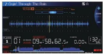
When in the slip mode, the currently playing position is indicated by a yellow line on the main unit display's waveform display (overall waveform or enlarged waveform). The position playing in the background is indicated by a white line on the main unit display's waveform display (overall waveform).
