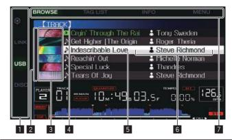
The indicator corresponding to the medium button that was pressed ([DISC], [USB], [LINK] or [rekordbox]) lights.
