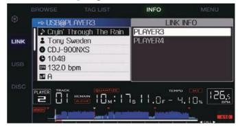
When another DJ player is connected by PRO DJ LINK, the details of the track loaded on the other DJ player can be checked.
