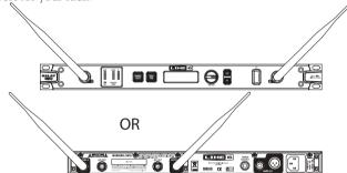
9. Antenna A/D & B/C Output Connectors (BNC) - Use the connectors to daisy chain multiple Relay G90 receivers. The outputs can be for Antenna A & B or C & D. It is user selectable which antennas get routed to the outputs. Be sure each additional receiver and its transmitter are set to a different channel.
