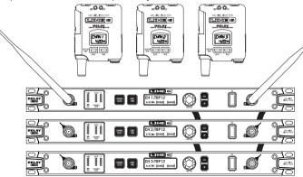
**Note:** Up to 6 G90 Receivers can be daisy-chained together when using external antennas. The last receiver in the chain should be "terminated" when linking receivers together.
