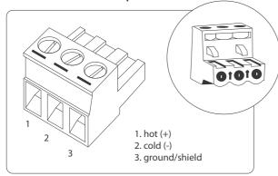
For output signals, connect a 4-pole (2-pole for CA601/1201/2401) Euroblock connector to the main output connector. Do NOT connect any terminal to ground. Do NOT connect the cold (-) terminals together for common returns. Make sure to set the Config switches in the correct position to match your intended use. Speaker wire of 14-18 AWG (0.8 to 2.5 mm) is recommended for connections up to 50 feet.
