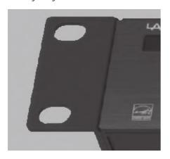
If your rack has rear rails, attach the rear flat brackets by reusing the screws from the chassis.
