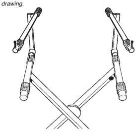
Place geared clamp 1 onto keyboard stand end tube. Using allen head screw 3 and locking nut 2, tighten clamp securely- see drawing.
