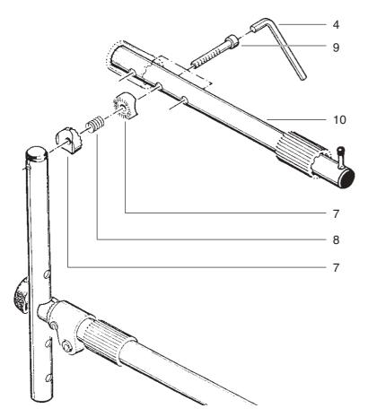
To assemble horizontal brace 10 and vertical support arm 5, align parts in sequence as illustrated and tighten- see drawing.
