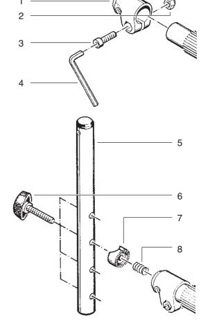
As illustrated connect vertical support arm 5 at desired height and tilt angle, to the locking device of the horizontal brace using locking knob 6, geared fastener 7 and spring 8; then tighten- see drawing.
