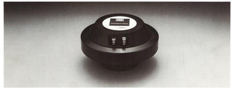
The model 2445J is a professional quality high frequency compression driver that incorporates JBL's newly developed titanium diamond diaphragm. The titanium diamond structure combines the ruggedness of phenolic and composite type diaphragms with the outstanding frequency response of aluminum and exotic metal diaphragms.
