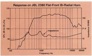
Frequency response of the 2445J coupled to a JBL 2380 Flat-Front Bi-Radial horn, measured on-axis at a distance of 1 meter with a 1-watt (4.0 V RMS) input in a reflection-free environment, with impedance vs. frequency curve. A horn with a pure exponential flare, such as typical radial horn designs, will exhibit greater high frequency output on-axis at the expense of lost angular coverage.
