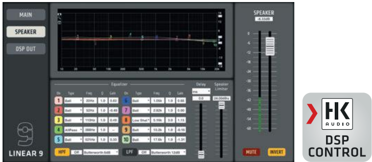
Screenshot of the remote DSP CONTROL software. You can download this software free of charge at the LINEAR 9 product page at www.hkaudio.com . The speaker and DSP Out parameters are identical, but the powerful onboard DSP lets you configure each set independently.
