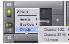
Routing a channel Direct Out to a plug-in in the Plug-Ins page
