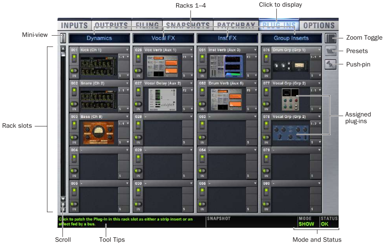
Figure 11. Plug-In racks and rack slots, Main view, with custom rack names shown.
