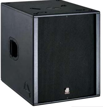
Made of multiplex coated with a robust black textured finish, the housing offers an M20 threaded shaft for a mounting pole, routed cups on the top panel designed to take another enclosure's feet for stacking, and threaded shafts on the rear panel that accept casters. A stable metal grille backed with laminated acoustic foam rubber protects the speakers.
