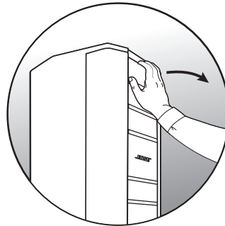
Pulling the array out
