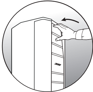
Pushing the array in
