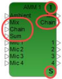
AMM Gated Block - Slave with mix and direct outputs
