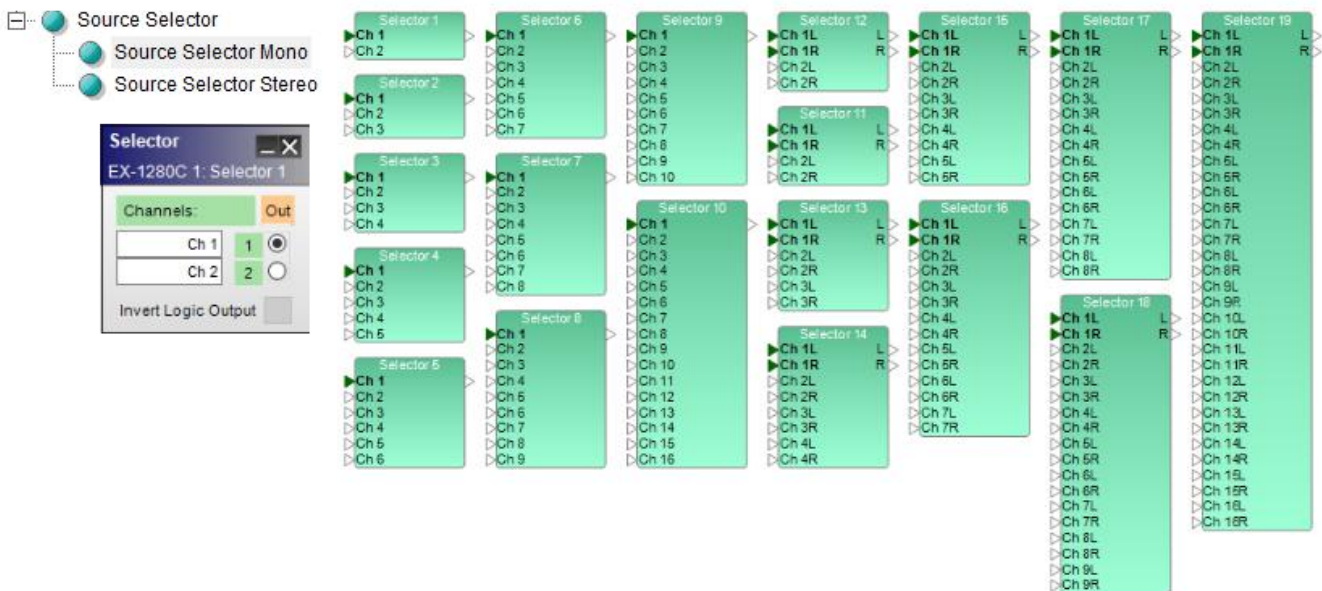
Source Selector processing blocks and mono - 2-channel control panel
