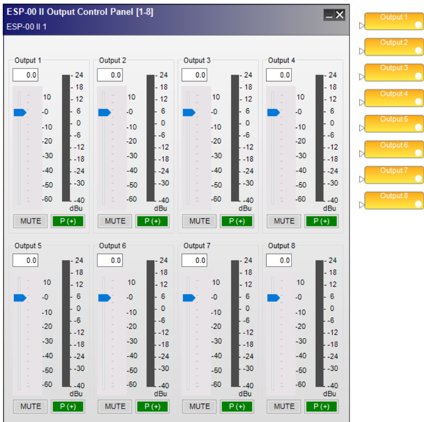
AES3 eight-channel output card control panel
