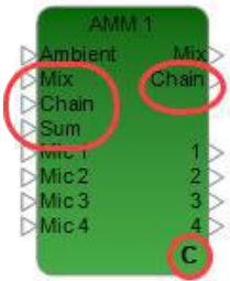
AMM Gated Block - CRC with mix and direct outputs
