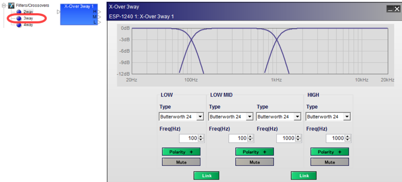
3-way crossover, processing block and control panel
