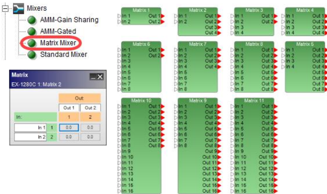
Matrix Mixer processing blocks and 2x2 control panel
