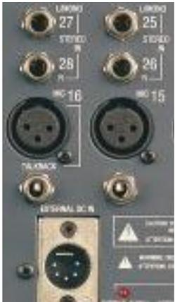
Stereo channels also accept separate mono mic inputs, so you don't waste channels when you're not working with stereo sources.
