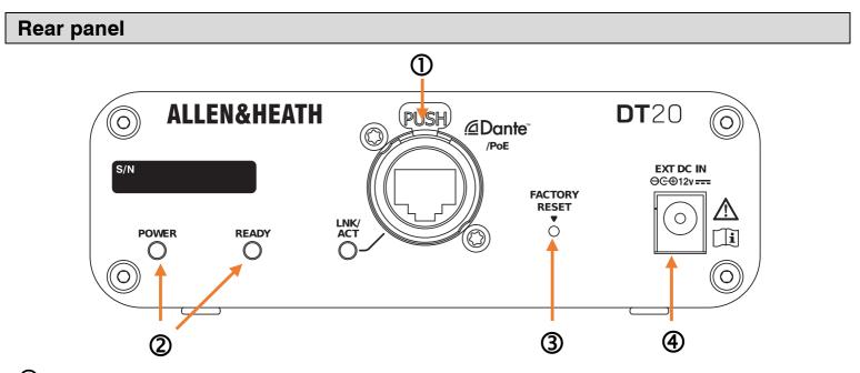
**Dante** EtherCon port for connection to the Dante network and Link / Activity LED indicator. Use a PoE Ethernet switch or PoE injector to power the unit via this port.
