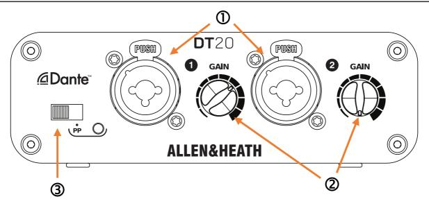
**(D)** Input sockets Balanced combi mic/line inputs. The TRS inputs have an integrated 20dB Pad for use with line level signals.
